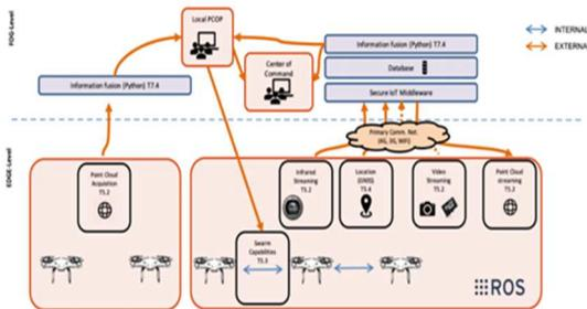
Fig. 3. Swarm of UAVs tasks during FASTER Project [14].
